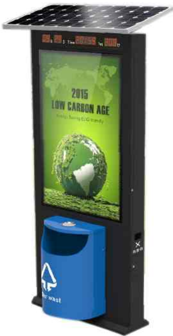
Model: HW-0039C Size: (L)1200x(W)1200x(H)2700(mm) Weight: Material:Stainless steel Solar Operate System Power: 18V80W Lithium Battery: 12V80AH LED System Power Consumption: LED/30W,
